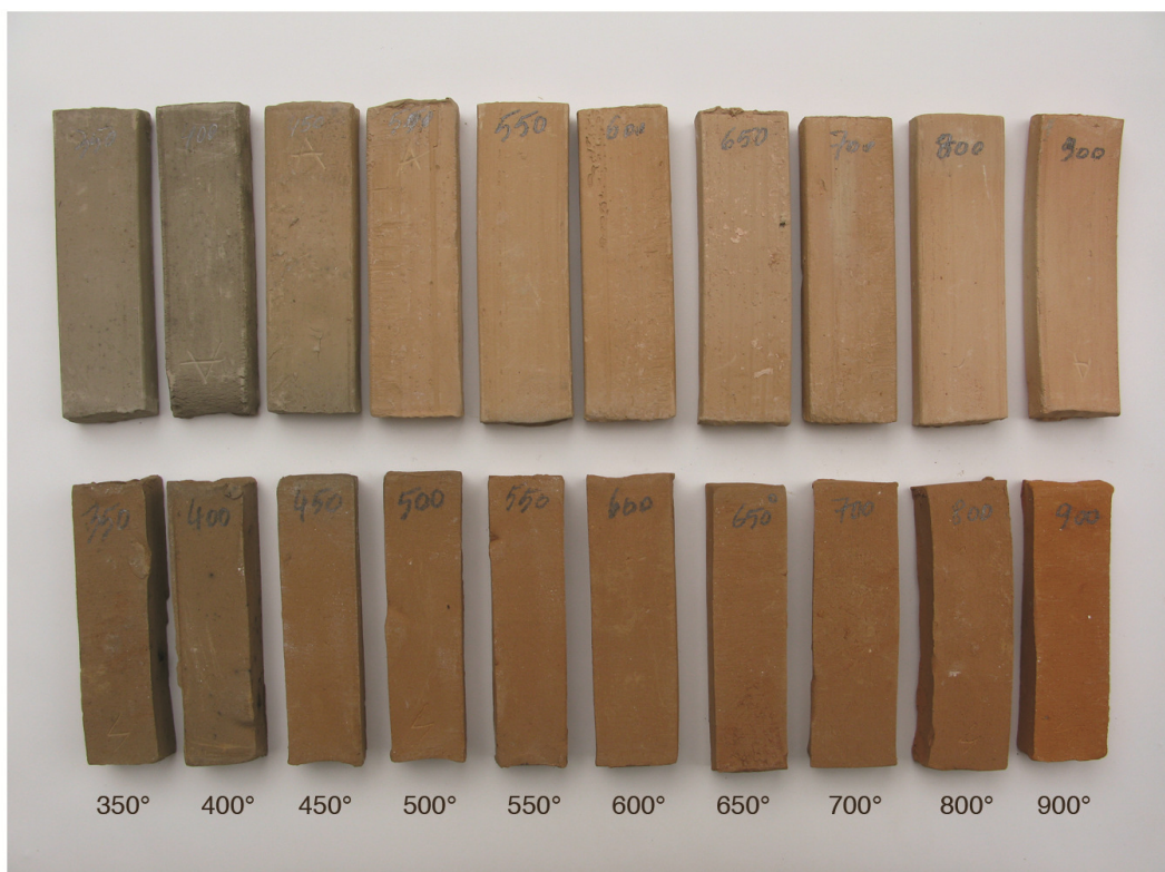
Fig.10 Clay test plates after firing. Temperature range between 350°C and 900°C.
